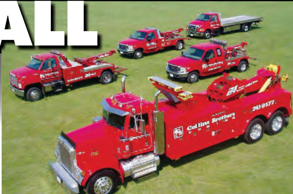
The majority of the towing equipment at Collins Brothers Towing is manufactured by Jerr-Dan. Pictured here clockwise from top left: an HPL 60 with a 1994 GMC chassis; an HPL35 with a 2002 Ford F450 chassis; a 21-ft. standard aluminum body carrier with a 2005 Ford F650 chassis; an HPL 35 with a 2001 Ford F350 chassis; and an HDL 500/280 25-ton wrecker with a 1999 Peterbilt chassis.
